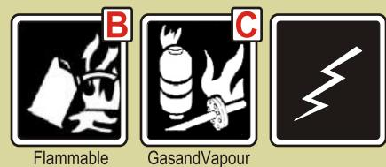
Flammable liquid fires      Gas and Vapour fires
